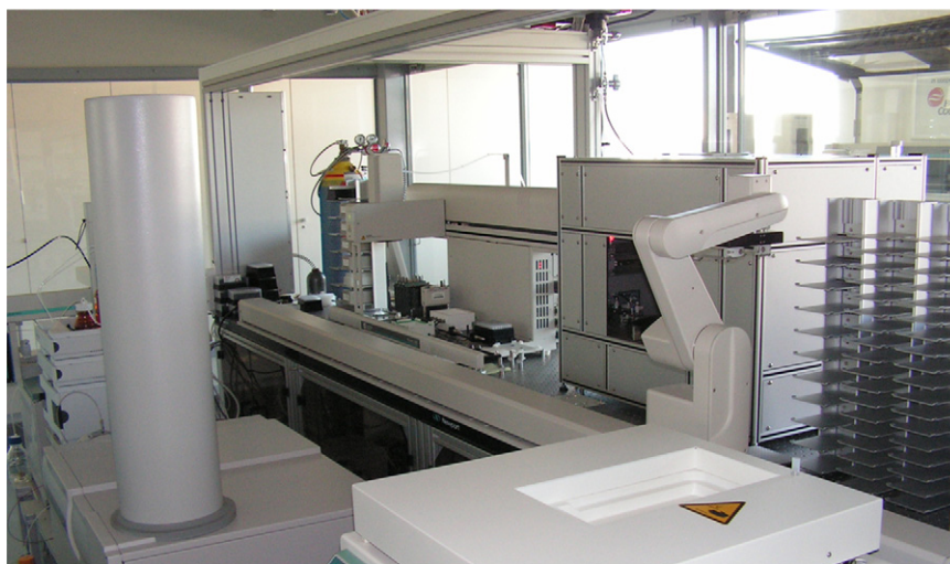
Fig. 5. Fully automated laboratory with high pressure microplate reactor, liquid handler, centrifuge and ESI-TOF-MS.
